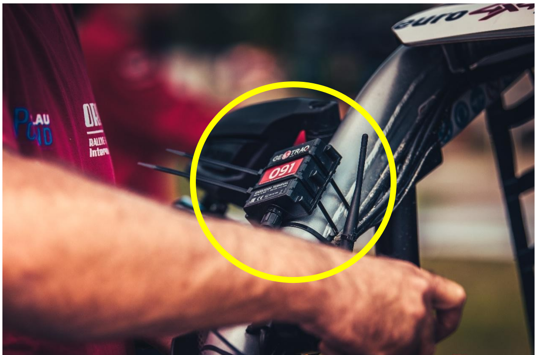
Installation of the GPS TRACKER on the roll cage "A-pillar" of a SSV using cable ties.
