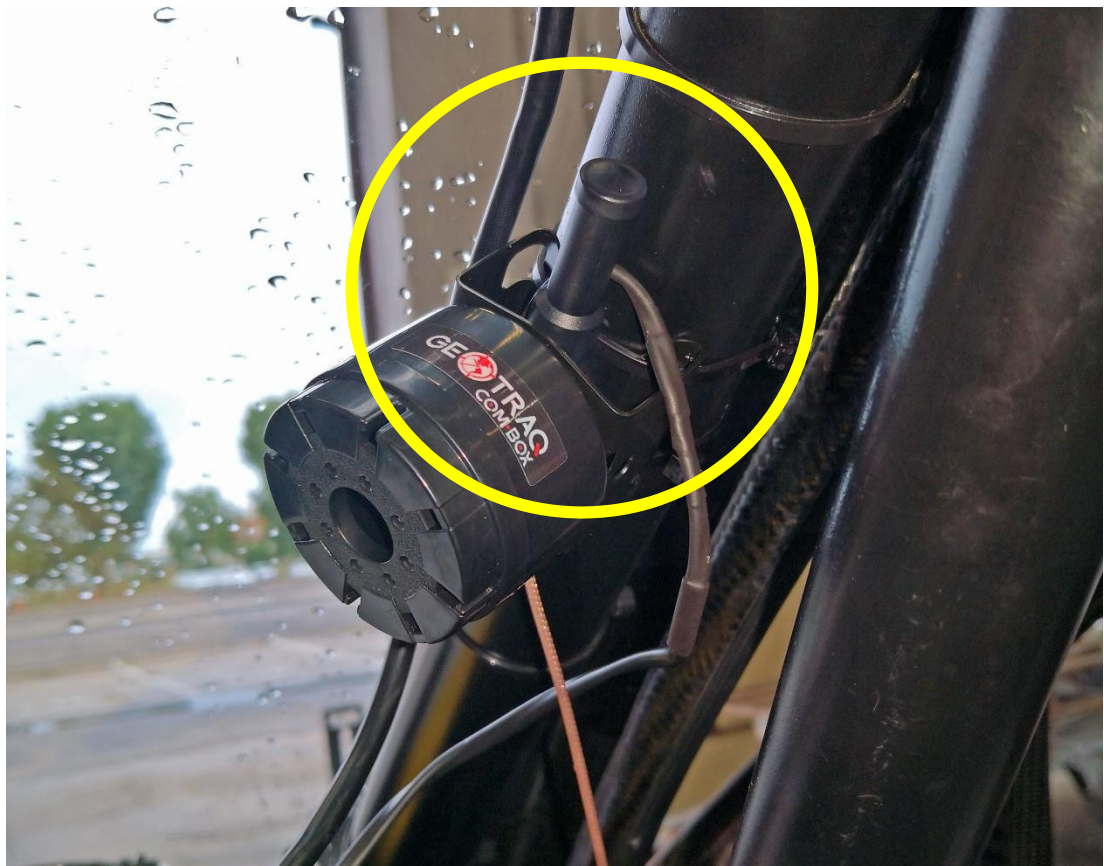
Installed antenna on the Buzzer unit (optional only when using extension cable).
