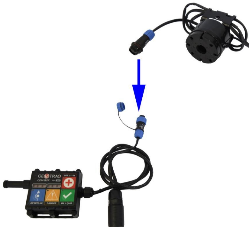
Connect the BUZZER to the COM-BOX.
