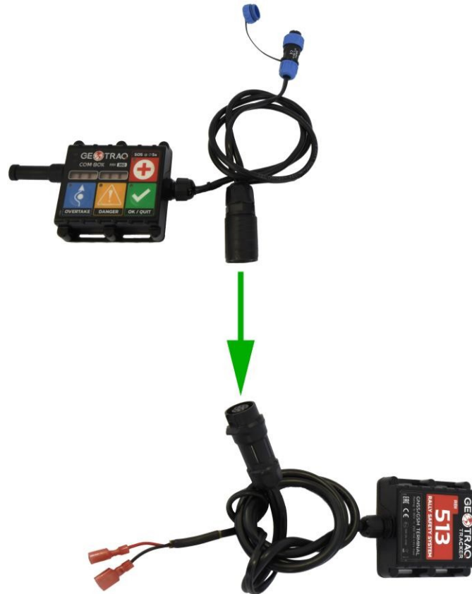
Connect the COM-BOX to the TRACKER.
