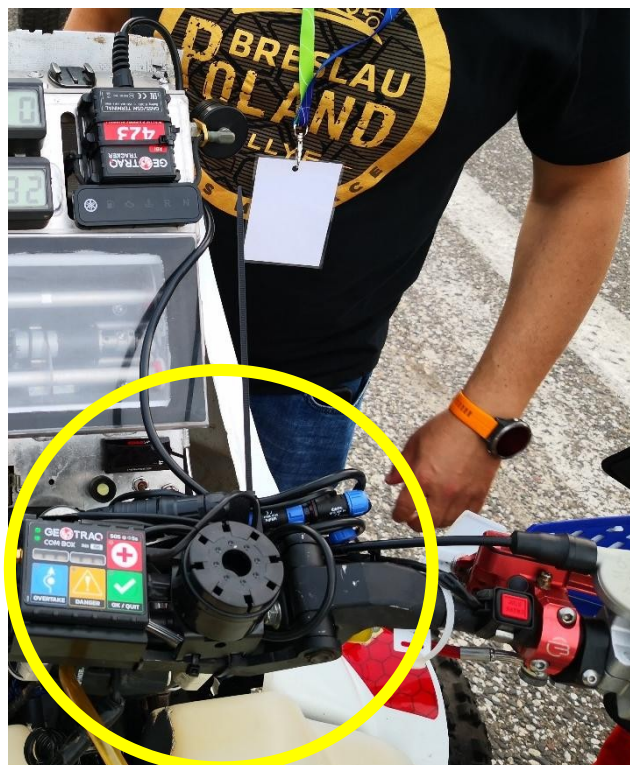
Installation of the Buzzer with bracket on the handle bar using cable ties.
