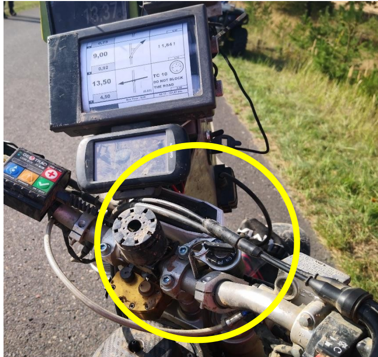
Installation of the Buzzer with bracket on the handle bar using cable ties.
