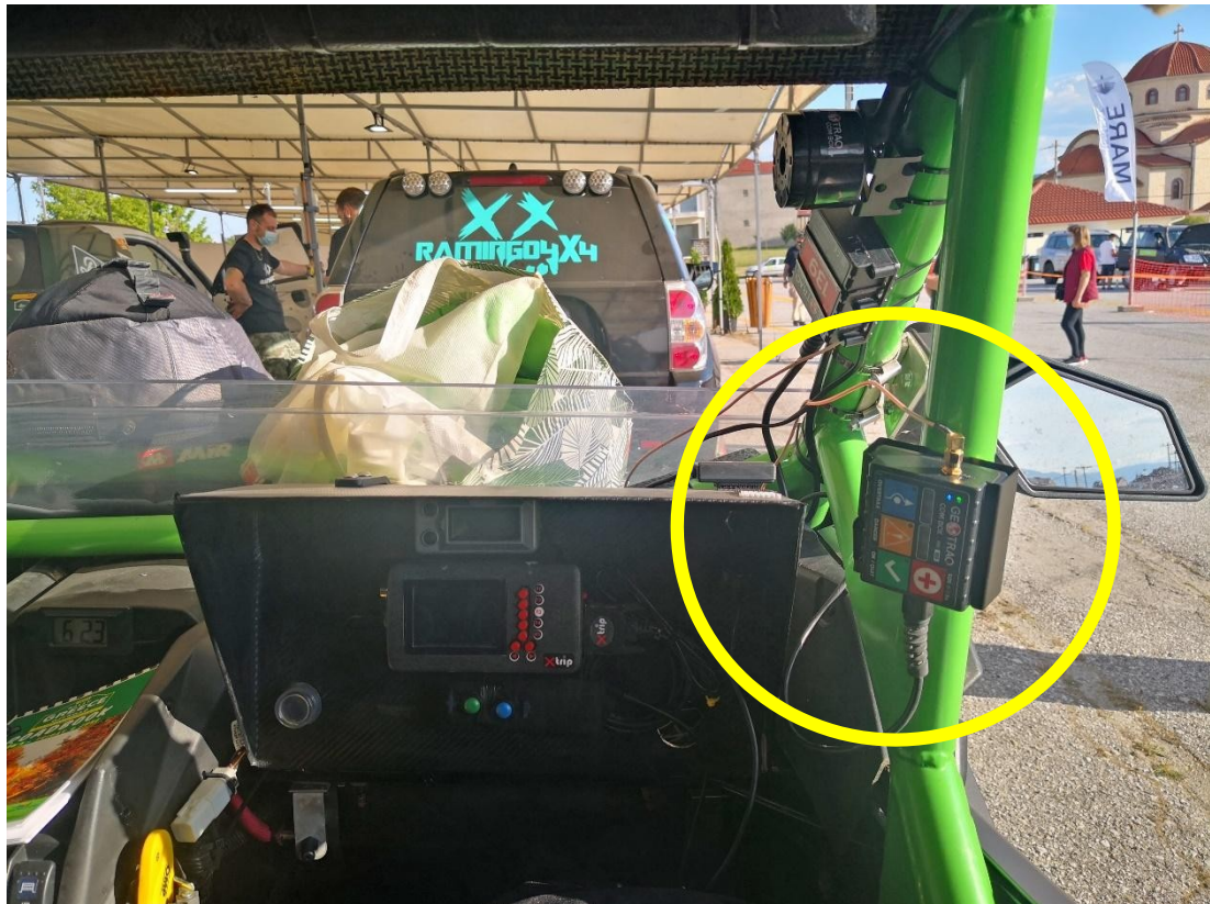
Installation of the Com-Box unit with bracket on the roll cage using cable ties. This must be in a CENTRAL location and not as indicated above, only in front of the co-driver.
