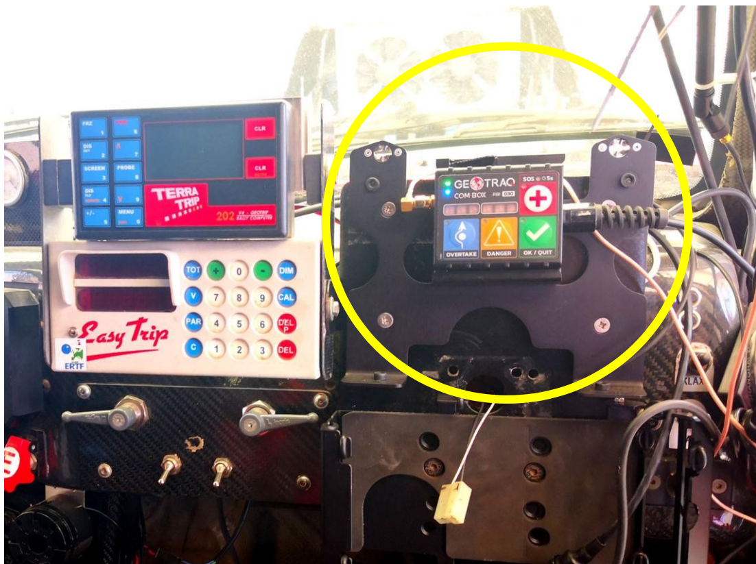
Installation of the Com-Box unit with bracket on the dashboard using bolts. This must be in a CENTRAL location and not as indicated above, only in front of the co-driver.
