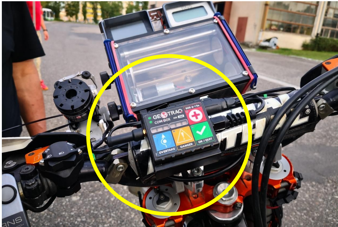
Installation of the Com-Box unit with bracket on the handle bar using cable ties.
